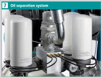
Compressors up to 160 kW are equipped with external separators that can be changed in a simple spin-off/spin-on process. Larger units have an internal separator cartridge. Due to the excellent separation efficiency of the system as a whole, the compressors can be used in the pressure range of 5.0 to 15.0 bar. Special pressures on request.
